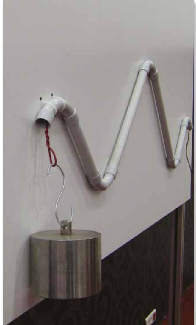
Slick cables can move through ducts even with small amount of force.
