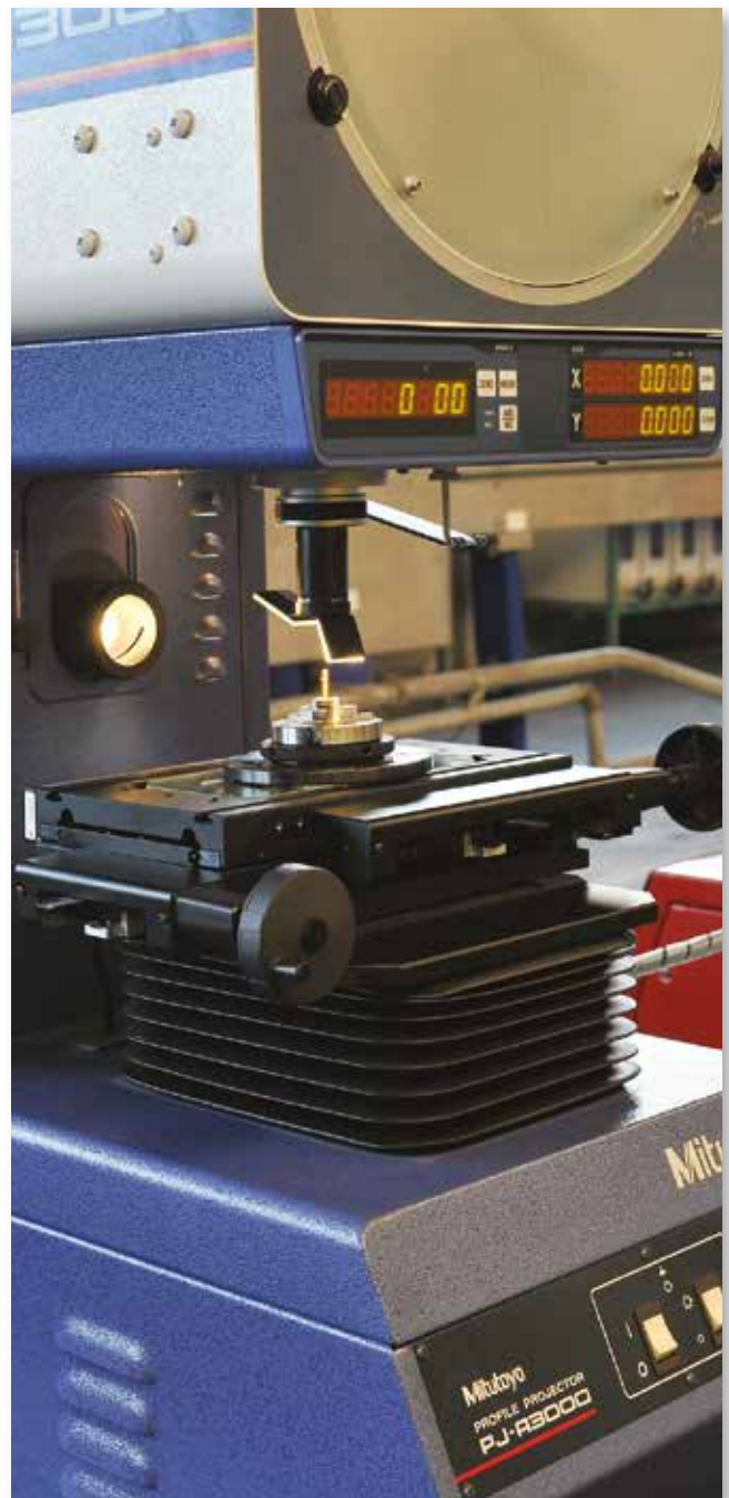
Geometric measurements are made using a profile projector.
